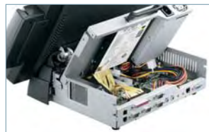
4. Easy to maintain and service Less than 4 screws to reach key components
